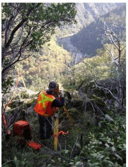
Our Surveying Coordinator, John Baker, surveys atop a cliff in the rugged South Yuba River Canyon. He is retracing the steps of Nineteenth Century surveyors using a highly capable, modern total station that is a precision transit, electronic distance measurer, and computer all in one. (Photo: Daniel Heinz)
